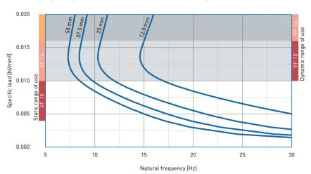
Natural frequency of a single-degree-offreedom system consisting of a fixed mass and an elastic bearing consisting of VIKAFOAM VF 10 on a stiff subgrade.
